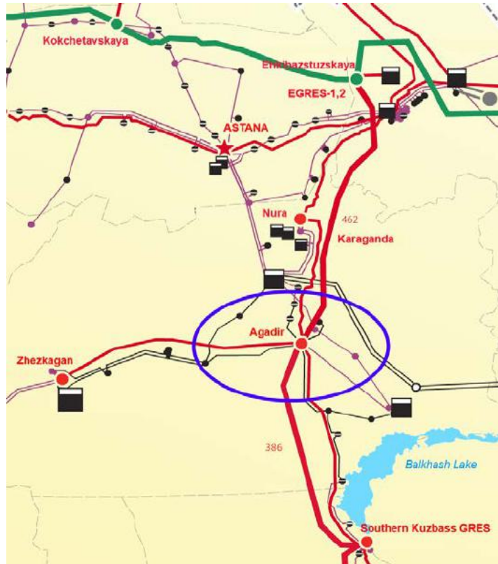
Figure 3. "North - South" 500 kV interconnection of the Republic of Kazakhstan
